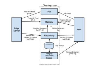
The Clearinghouse is composed of several IHE defined actors and participates in different transactions with the Edge Server and PHR. In the model shown above, the internals of the Clearinghouse are shown for illustrative purposes. The implementation requirements are defined by the exchanges with the Edge Server and PHR systems.
